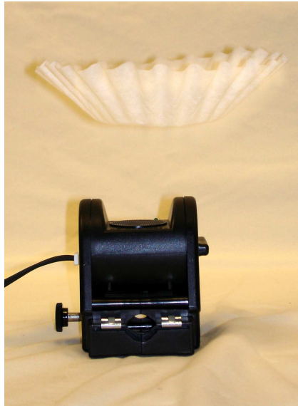
Figure 3.3: A falling coffee filter does not fall with constant acceleration due to the effects of air resistance. The motion sensor below the filter is connected to a computer, which records position data and stores it in a text file.
