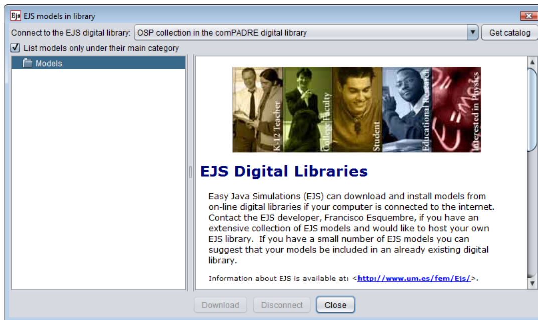
Figure 1.4: The Digital Libraries window of EJS . Select one of the available repositories using the combo box at the top of the window and click the Get catalog button to retrieve the list of available models.
